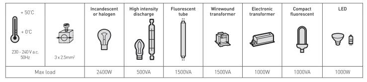
Note: When a small high impedance load is connected (e.g. a single LED or compact fluorescent lamp), the load may flicker when it is supposed to be OFF due to the small amount of current required to power the PE170/10. This can be fixed by connecting a ELE6VA Load Correction Network in parallel with the load, so as to provide an alternate current path. The larger the load, the smaller the chance of this issue occurring.
